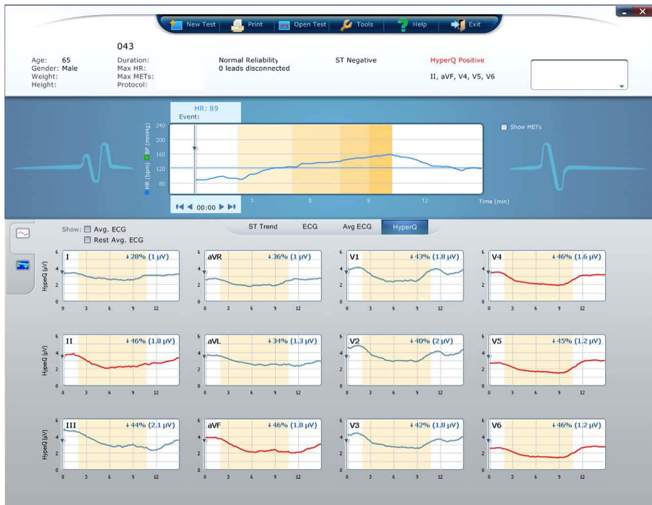
Fig. 2. Heart rate (top panel) and time-intensity curves of HFQRS components for all 12 leads obtained in an ischemic patient during exercise. Absolute (in microvolt) and relative (in percentage) HFQRS intensity reductions are indicated for each lead. Leads that exhibit significant HFQRS reduction are presented in red, whereas those with less pronounced reduction are presented in blue. In this patient, 5 leads were found indicative of ischemia, therefore suggesting the presence of ischemic heart disease. See text for details. (Available in color online at www.sciencedirect.com and www.jecgonline.com ).
